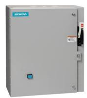
Non-reversing motor starter, Size 1, Three phase full voltage, Solid-state overload relay, OLR amp range 5.5-22A, 24VDC coil, Combination type, 30A non-fusible disconnect, Enclosure NEMA type 1, Indoor general purpose use, Extra-wide enclosure
