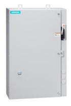
Non-reversing motor starter, Size 1, Three phase full voltage, Solid-state overload relay, OLR amp range 3-12A, 24VAC 50-60Hz coil, Combination type, 30A non-fusible disconnect, Encl NEMA type 4X 304 S-Steel, Water/dust tight noncorrosive, Extra-wide enclosure
