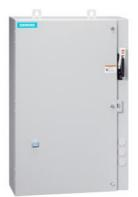
Non-reversing motor starter, Size 1, Three phase full voltage, Solid-state overload relay, OLR amp range 3-12A, Combination type, 30A fusible disconnect, 30A/600V fuse clip, Enclosure NEMA type 4/12, Water/dust tight for outdoors, Extra-wide enclosure
