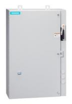
Non-reversing motor starter, Size 1, Three phase full voltage, Solid-state overload relay, OLR amp range 3-12A, Combination type, 30A fusible disconnect, 30A/250V fuse clip, Enclosure NEMA type 4/12, Water/dust tight for outdoors, Extra-wide enclosure
