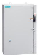
Non-reversing motor starter, Size 1, Three phase full voltage, Solid-state overload relay, OLR amp range 0.75-3.4A, 24VAC 50-60Hz coil, Combination type, 30A fusible disconnect, 30A/250V fuse clip, Encl NEMA type 4X 304 S-Steel, Water/dust tight noncorrosive, Extra-wide enclosure
