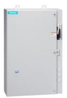
Non-reversing motor starter, Size 1, Three phase full voltage, Solid-state overload relay, OLR amp range 0.75-3.4A, 208VAC 60Hz coil, Combination type, 30A non-fusible disconnect, Enclosure NEMA type 4/12, Water/dust tight for outdoors, Extra-wide enclosure
