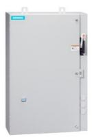
Non-reversing motor starter, Size 1, Three phase full voltage, Solid-state overload relay, OLR amp range 0.75-3.4A, Combination type, 30A non-fusible disconnect, Enclosure NEMA type 4/12, Water/dust tight for outdoors, Extra-wide enclosure
