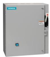
Non-reversing motor starter, Size 1, Three phase full voltage, Solid-state overload relay, OLR amp range 0.75-3.4A, 24VDC coil, Combination type, 30A non-fusible disconnect, Enclosure NEMA type 1, Indoor general purpose use, Extra-wide enclosure
