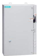
Non-reversing motor starter, Size 1, Three phase full voltage, Solid-state overload relay, OLR amp range 0.25-1A, Combination type, 30A fusible disconnect, 30A/250V fuse clip, Encl NEMA type 4X 304 S-Steel, Water/dust tight noncorrosive, Extra-wide enclosure
