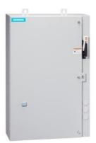
Non-reversing motor starter, Size 1, Three phase full voltage, Solid-state overload relay, OLR amp range 0.25-1A, 110V 50Hz / 120V 60Hz coil, Combination type, 30A non-fusible disconnect, Encl NEMA type 4X 304 S-Steel, Water/dust tight noncorrosive, Extra-wide enclosure
