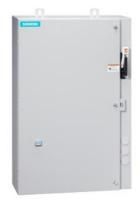
Non-reversing motor starter, Size 1, Three phase full voltage, Solid-state overload relay, OLR amp range 0.25-1A, 208VAC 60Hz coil, Combination type, 30A fusible disconnect, 30A/600V fuse clip, Encl NEMA type 4X 304 S-Steel, Water/dust tight noncorrosive, Extra-wide enclosure
