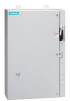
Non-reversing motor starter, Size 1, Three phase full voltage, Solid-state overload relay, OLR amp range 0.25-1A, 208VAC 60Hz coil, Combination type, 30A fusible disconnect, 30A/600V fuse clip, Enclosure NEMA type 4/12, Water/dust tight for outdoors, Extra-wide enclosure
