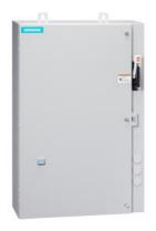
Non-reversing motor starter, Size 0, Three phase full voltage, Solid-state overload relay, OLR amp range 5.5-22A, 24VDC coil, Combination type, 30A non-fusible disconnect, Enclosure NEMA type 4/12, Water/dust tight for outdoors, Extra-wide enclosure
