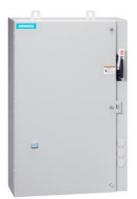
Non-reversing motor starter, Size 0, Three phase full voltage, Solid-state overload relay, OLR amp range 3-12A, 24VAC 50-60Hz coil, Combination type, 30A non-fusible disconnect, Encl NEMA type 4X 304 S-Steel, Water/dust tight noncorrosive, Extra-wide enclosure
