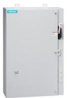
Non-reversing motor starter, Size 0, Three phase full voltage, Solid-state overload relay, OLR amp range 3-12A, 24VDC coil, Combination type, 30A fusible disconnect, 30A/600V fuse clip, Enclosure NEMA type 4/12, Water/dust tight for outdoors, Extra-wide enclosure
