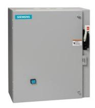
Non-reversing motor starter, Size 0, Three phase full voltage, Solid-state overload relay, OLR amp range 3-12A, 240V 50Hz / 277V 60Hz coil, Combination type, 30A non-fusible disconnect, Enclosure NEMA type 1, Indoor general purpose use, Extra-wide enclosure
