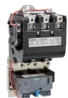
Non-reversing motor starter Size 4 Three phase full voltage Solid-state overload relay OLRelay amp range 50-200A 24VAC 50-60HZ coil Combination type No enclosure
