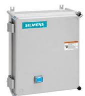
Non-reversing motor starter, Size 3 1/2, Three phase full voltage, Solid-state overload relay, OLR amp range 50-200A, Non-combination type, Enclosure type 4X fiberglass, Water/dust tight noncorrosive, Standard width enclosure
