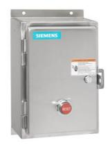
Non-reversing motor starter, Size 3 1/2, Three phase full voltage, Amb. compensate bimetal OLR, Contactor amp rating 115A, 24VAC 50-60Hz coil, Noncombination type, Encl. type 4X 304 S. Steel, Water/dust tight noncorrosive
