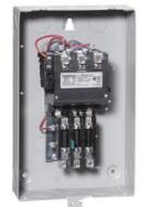
Non-reversing motor starter, Size 3 1/2, Three phase full voltage, Amb. compensate bimetal OLR, Contactor amp rating 115A, Non-combination type, Enclosure type 1, Indoor general purpose use
