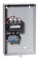
Non-reversing motor starter, Size 3, Three phase full voltage, Solid-state overload relay, OLR amp range 25-100A, 24VDC coil, Non-combination type, Enclosure type 1, Indoor general purpose use, Standard width enclosure
