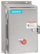
Non-reversing motor starter Size 2 1/2 Three phase full voltage Solid-state overload relay OLRelay amp range 25-100A 190-220/220-240V 50/60HZ coil Combination type Water/dust tight non-corrosive
