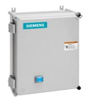
Non-reversing motor starter, Size 2 1/2, Three phase full voltage, Solid-state overload relay, OLR amp range 25-100A, 24VDC coil, Non-combination type, Enclosure type 4X fiberglass, Water/dust tight noncorrosive, Standard width enclosure
