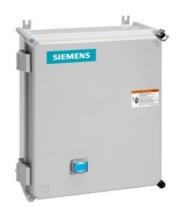
Non-reversing motor starter, Size 2 1/2, Three phase full voltage, Solid-state overload relay, OLR amp range 25-100A, 24VAC 50-60Hz coil, Non-combination type, Enclosure type 4X fiberglass, Water/dust tight noncorrosive, Standard width enclosure
