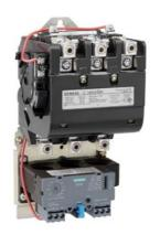
Non-reversing motor starter Size 2 1/2 Three phase full voltage Solid-state overload relay OLRelay amp range 25-100A 24VAC 50-60HZ coil Combination type No enclosure
