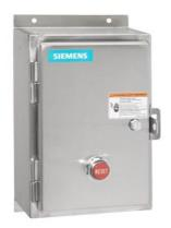
Non-reversing motor starter, Size 2 1/2, Three phase full voltage, Amb. compensate bimetal OLR, Contactor amp rating 60A, 240V 50Hz / 277V 60Hz coil, Non-combination type, Encl. type 4X 304 S. Steel, Water/dust tight noncorrosive
