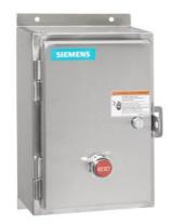
Non-reversing motor starter, Size 2 1/2, Three phase full voltage, Amb. compensate bimetal OLR, Contactor amp rating 60A, Non-combination type, Encl. type 4X 304 S. Steel, Water/dust tight noncorrosive
