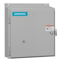
Non-reversing motor starter, Size 2 1/2, Three phase full voltage, Amb. compensate bimetal OLR, Contactor amp rating 60A, 24VAC 50-60Hz coil, Noncombination type, Enclosure type 12, Dust/drip proof for indoors
