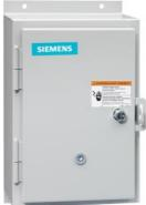
Non-reversing motor starter, Size 1 3/4, Three phase full voltage, Solid-state overload relay, OLRelay amp range 10-40a, 190 220/220 240V 50/60HZ coil, Non-combination type, Enclosure type 12, Dust/drip proof for indoors, Extra-wide enclosure
