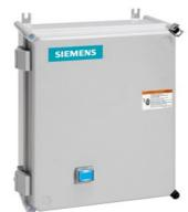
Non-reversing motor starter, Size 1 3/4, Three phase full voltage, Solid-state overload relay, OLR amp range 10-40A, 110V 50Hz / 120V 60Hz coil, Non-combination type, Enclosure type 4X fiberglass, Water/dust tight noncorrosive, Standard width enclosure
