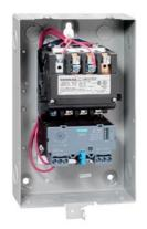
Non-reversing motor starter, Size 1 3/4, Three phase full voltage, Solid-state overload relay, OLR amp range 10-40A, 24VDC coil, Non-combination type, Enclosure type 1, Indoor general purpose use, Standard width enclosure
