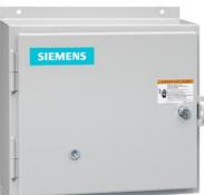
Non-reversing motor starter, Size 1 3/4, Three phase full voltage, Solid-state overload relay, OLR amp range 10-40A, Non-combination type, Enclosure type 12, Dust/drip proof for indoors, Standard width enclosure
