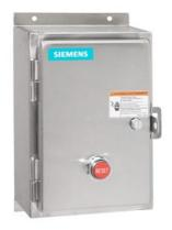
Non-reversing motor starter Size 1 Three phase full voltage Solid-state overload relay OLRelay amp range 10-40a 110VAC 50HZ / 120VAC 60HZ coil Combination type Water/dust tight non-corrosive
