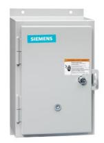
Non-reversing motor starter, Size 1, Three phase full voltage, Solid-state overload relay, OLRelay amp range 10-40a, 24VAC 50-60HZ coil, Non-combination type, Enclosure type 12, Dust/drip proof for indoors, Extra-wide enclosure
