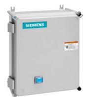
Non-reversing motor starter, Size 1, Three phase full voltage, Solid-state overload relay, OLR amp range 10-40A, 24VAC 50-60Hz coil, Non-combination type, Enclosure type 4X fiberglass, Water/dust tight noncorrosive, Standard width enclosure
