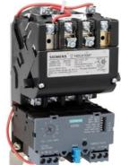
Non-reversing motor starter Size 1 Three phase full voltage Solid-state overload relay OLRelay amp range 10-40a 240VAC 50HZ / 277VAC 60HZ coil Combination type No enclosure
