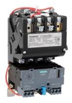
Non-reversing motor starter Size 1 Three phase full voltage Solid-state overload relay OLRelay amp range 10-40a 220-240/440-480VAC 60HZ coil Combination type No enclosure
