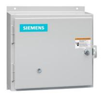
Non-reversing motor starter, Size 1, Three phase full voltage, Solid-state overload relay, OLR amp range 10-40A, 208VAC 60Hz coil, Non-combination type, Enclosure type 12, Dust/drip proof for indoors, Standard width enclosure
