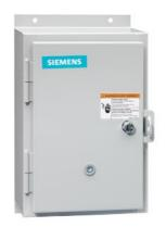
Non-reversing motor starter, Size 1, Three phase full voltage, Solid-state overload relay, OLRelay amp range 5.5-22a, 380 440/440 480V 50/60HZ coil, Non-combination type, Enclosure type 12, Dust/drip proof for indoors, Extra-wide enclosure
