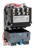
Non-reversing motor starter Size 1 Three phase full voltage Solid-state overload relay OLRelay amp range 5.5-22A 208VAC 60HZ coil Combination type No enclosure
