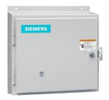
Non-reversing motor starter, Size 1, Three phase full voltage, Solid-state overload relay, OLRelay amp range 5.5-22a, 550/575 600 50/60HZ coil, Non-combination type, Enclosure type 12, Dust/drip proof for indoors, Standard width enclosure
