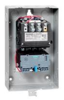
Non-reversing motor starter, Size 1, Three phase full voltage, Solid-state overload relay, OLR amp range 3-12A, Non-combination type, Enclosure type 1, Indoor general purpose use, Standard width enclosure
