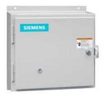
Non-reversing motor starter, Size 1, Three phase full voltage, Solid-state overload relay, OLRelay amp range 3-12a, 240V 50HZ / 277V 60HZ coil, Non-combination type, Enclosure type 12, Dust/drip proof for indoors, Standard width enclosure
