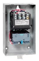
Non-reversing motor starter Size 1 Single phase full voltage Solid-state overload relay OLRelay amp range 3-12A 190-220/220-240V 50/60HZ coil Combination type Indoor general purpose use
