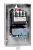
Non-reversing motor starter, Size 1, Single phase full voltage, Solid-state overload relay, OLR amp range 3-12A, 110V 50Hz / 120V 60Hz coil, Non-combination type, Enclosure type 1, Indoor general purpose use, Standard width enclosure
