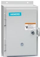
Non-reversing motor starter, Size 1, Three phase full voltage, Solid-state overload relay, OLRelay amp range 0.75-3.4a, 24VAC 50-60HZ coil, Non-combination type, Enclosure type 12, Dust/drip proof for indoors, Extra-wide enclosure
