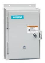
Non-reversing motor starter, Size 1, Three phase full voltage, Solid-state overload relay, OLRelay amp range 0.75-3.4a, 190 220/220 240V 50/60HZ coil, Non-combination type, Enclosure type 12, Dust/drip proof for indoors, Extra-wide enclosure
