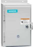
Non-reversing motor starter, Size 1, Three phase full voltage, Solid-state overload relay, OLRelay amp range 0.75-3.4a, 220 240/440 480VAC 60HZ coil, Non-combination type, Enclosure type 12, Dust/drip proof for indoors, Extra-wide enclosure
