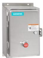
Non-reversing motor starter, Size 1, Three phase full voltage, Solid-state overload relay, OLR amp range 0.75-3.4A, 110V 50Hz / 120V 60Hz coil, Non-combination type, Encl. type 4X 304 S. Steel, Water/dust tight noncorrosive, Standard width enclosure
