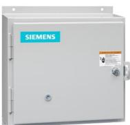
Non-reversing motor starter, Size 1, Three phase full voltage, Solid-state overload relay, OLR amp range 0.75-3.4A, 110V 50Hz / 120V 60Hz coil, Non-combination type, Enclosure type 12, Dust/drip proof for indoors, Standard width enclosure
